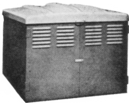
Figure 1-5(g) Steel hose house of compact dimensions for installation over a private hydrant. House is shown closed. Top lifts up and doors on front side open for complete accessibility.
