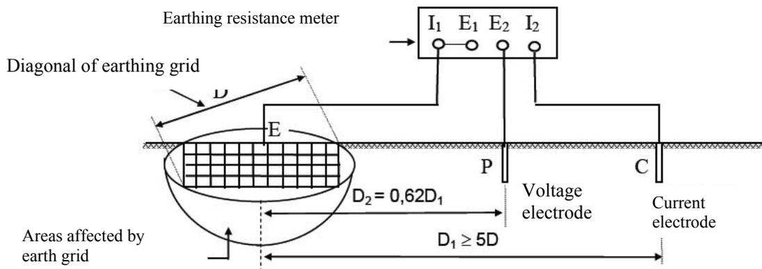
**Figure A.3: Metering circuit of earthing resistance of earth grid or earth electrodes**
