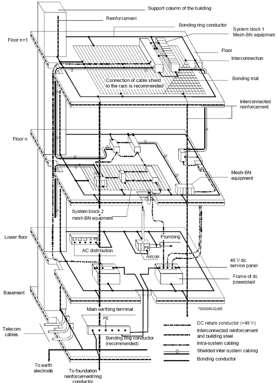
Figure 2: Mesh – bonding network (M-BN) inside a telecommunication building
