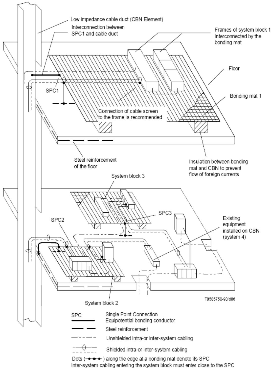
**Figure 3: Mesh – Isolated bonding network (M-IBN) inside a telecommunication building**
