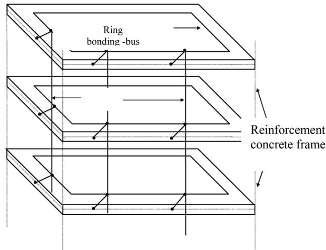
**Figure 1: Common bonding network (CBN) inside a telecommunication building**
