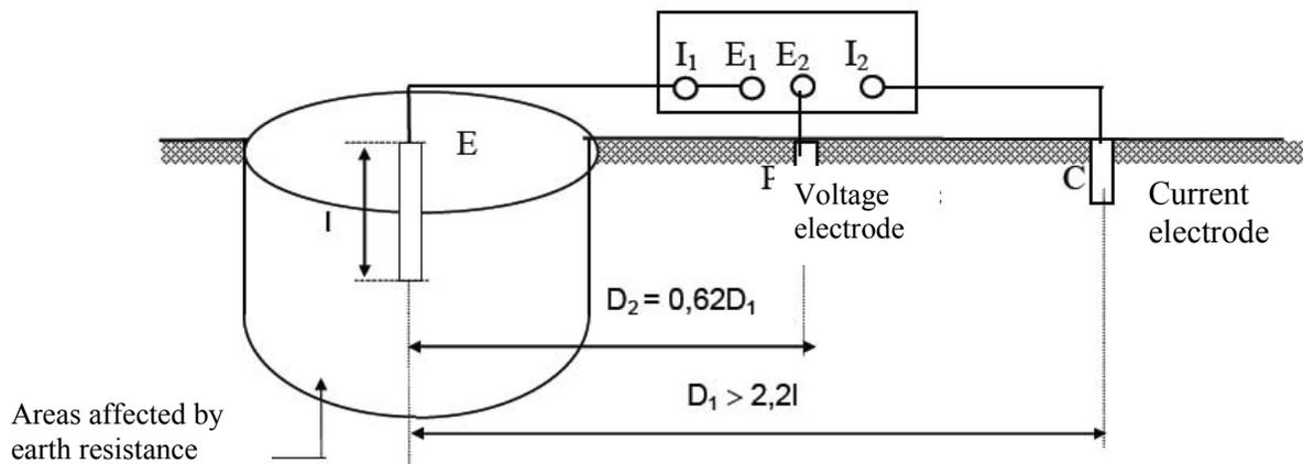
**Figure A.2: Metering circuit of earthing resistance of vertical earthing electrode**
