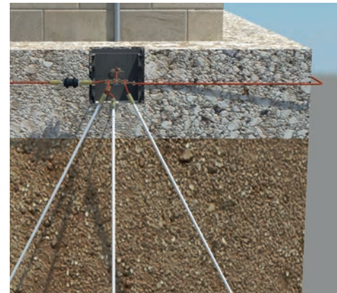
Fig. 13 – Grounding System cross section.
