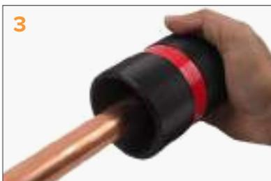
Remove internal and external burrs from the tube. (Fig. 3)
