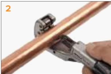
Ensure that the tube end is cut square and remains round. (Fig. 2)
