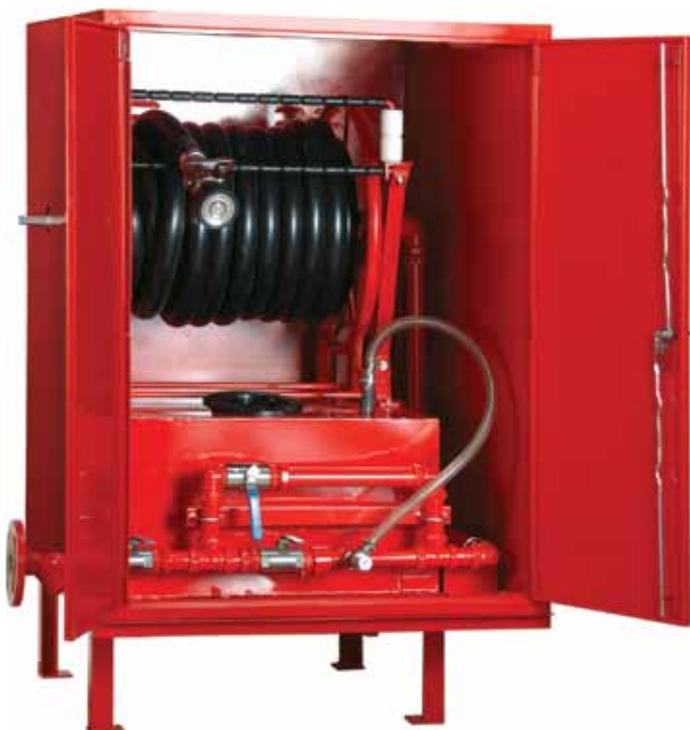
This hose reel station is complete with 1-1/2" x 30M rigid hose, 225L AFFF foam, stainless steel foam concentrate storage tank, 95GPM foam inductor and nozzle. A bypass loop is provided for water or foam discharge.
