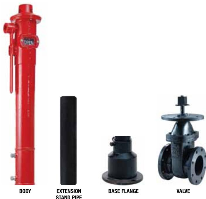
The Indicator Post with gate valve provides a means for operating a buried or otherwise inaccessible gate valve to controlled flow of water in buried pipe. A wrench is provided to fit on top of the unit for turning the gate valve open and shut.
