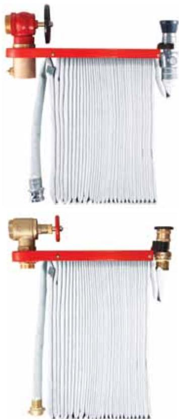
SRI's hose rack assembly is located inside buildings at the wet or dry riser outlet. It features a rack in which hangs the layflat fire hose (30m). An automatic release mechanism allows water to flow through the hose after removal of the hose and nozzle. The rack is available in sizes of 1-1/2" and 2-1/2". There are two methods of mounting the hose rack. One is by using a wall bracket and the other is by fixing on to a right angle valve.
