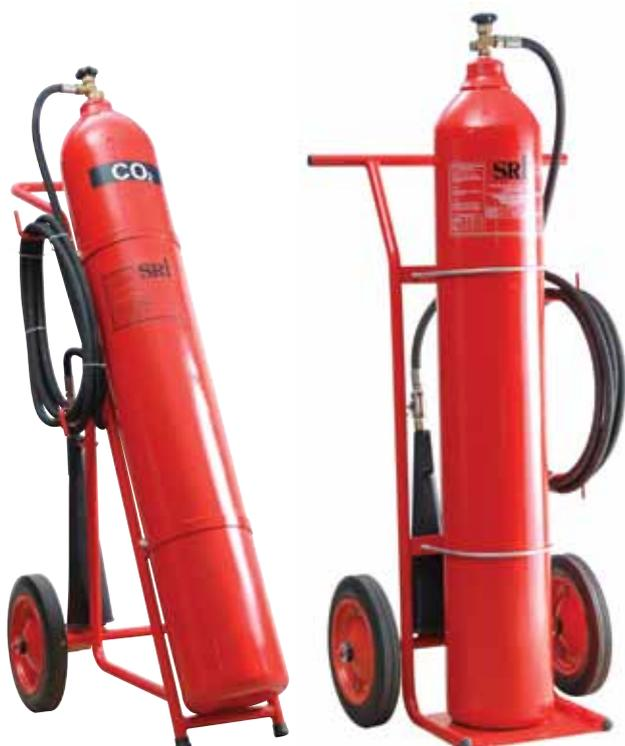
Carbon dioxide fire extinguisher on trolley is made of seamless Manganese steel to withstand high storage pressure. It is effective on class B and class C fires and electrically non conductive.
