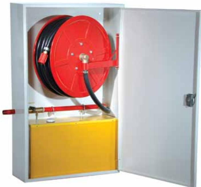
Foam hose reel is complete with a foam inductor used to supply mixture of foam concentrate and water. Foam solution is most effective for extinguisher fire involving flammable liquid such as petrol and solvents.
