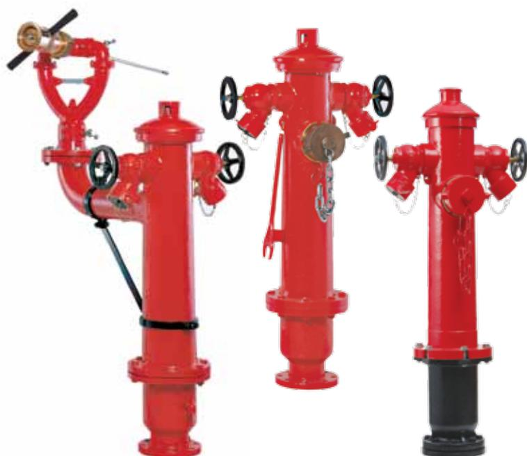
This hydrant is operated by using a hydrant wrench to turn the operating mechanism at the top of the hydrant which will open the valve seat. It is available in two sizes 4" and 6".
