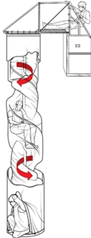
Vertical-Spiral Escape Chute is a device which emergency in the crowd and rapid evacuation of people from high structures, where one chute is capable of evacuating some evacuees from a high rise building in 15 to 20 minutes. It is also possible for a person to enter the chute, and then have an evacuee second person placed upon their shoulders, to assist the second person to evacuate.
