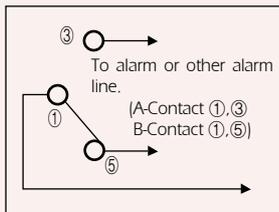
**Pressure Switch Wiring**
