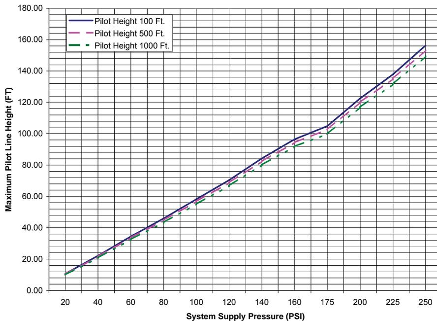
**Figure 4 - 4" (DN100) Model F-1 Deluge Valves**
