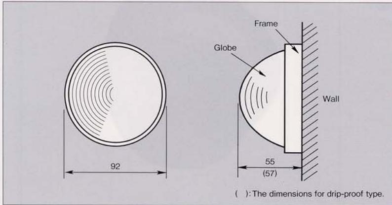
The location lamp has a high luminance with which the light can be clearly visible at a position 10m apart from the location lamp along with a direction of an angle of 15° or more from the mounting surface.
