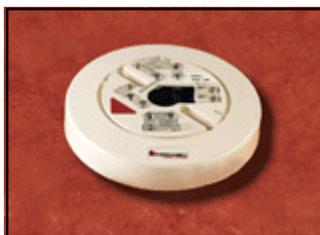
The HSC-4R is designed specifically for 24 volt 4 wire applications using HOCHIKI NS Conventional Models SIJ-24 Ionization Smoke Detector, SLR-24 Photoelectric Smoke Detector, SLR-24H Photoelectric with Heat Smoke Detector, SLR-835 Photoelectric Smoke Detector, or DCD-135/190 Fixed Temperature/Rate-of-Rise Heat Detector. The 6" diameter base is current limited. A direct short occurs across the loop when the detector is actuated.
