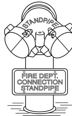
**4-3.4\*** When pumping to a fire department standpipe connection, the pump operator should consider the following factors when calculating pump discharge pressure:
