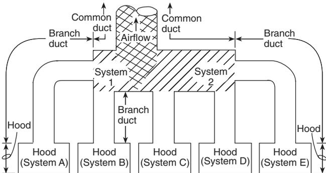
**Figure A-7-3.4(c)** Independent operation of systems that protect only the common exhaust duct.
