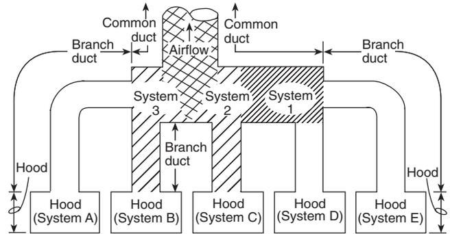
**Figure A-7-3.4(f) Independent operation of (a) a combination of a system that protects only a portion of the common exhaust duct and (b) cooking appliance, hood, and branch duct systems, two or more of which protect the remainder of the common exhaust ducts.**
