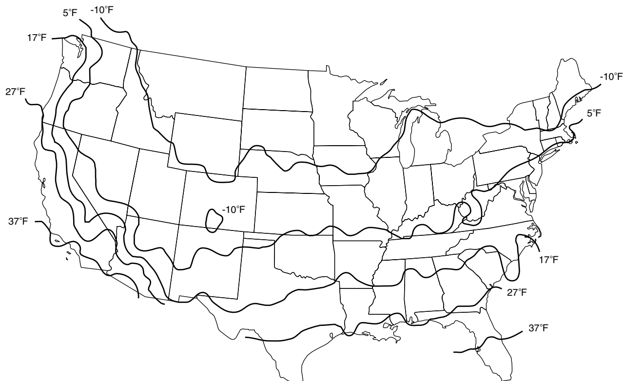
Figure G.19 Range of winter design temperatures were used in analyzing exterior masonry chimneys in the United States.
