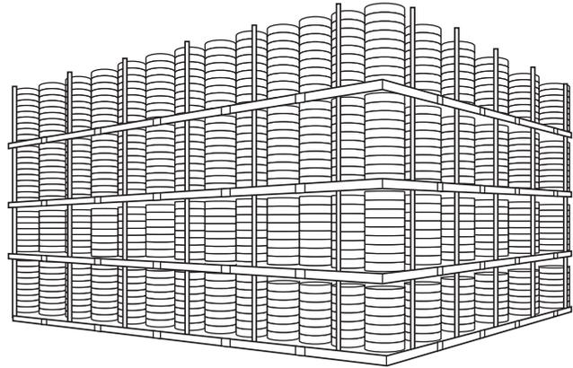
Figure 6-2(f) On-tread, on-floor tire storage arrangement (normally banded).
