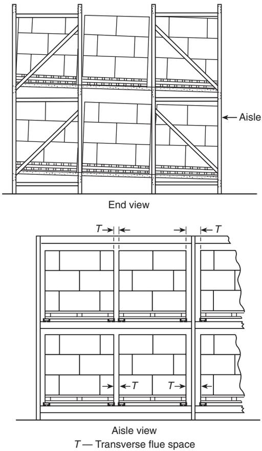
Figure A-5-3.1(c)(3) Drive-in rack — two or more pallets deep (fork truck drives into the rack to deposit and withdraw loads in the depth of the rack).
