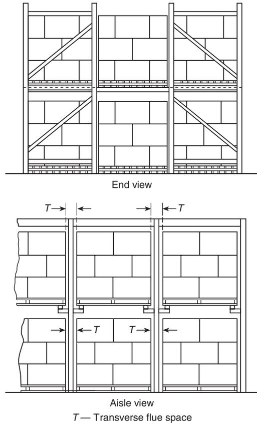
Figure A-5-3.1(c)(4) Flow-through rack.
