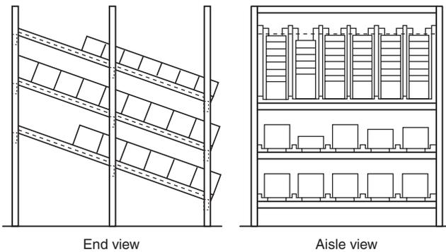
Figure A-5-3.1(c)(5) Portable racks.
