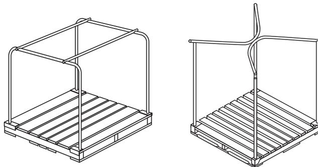
Figure 6-2(c) Open portable tire rack.
