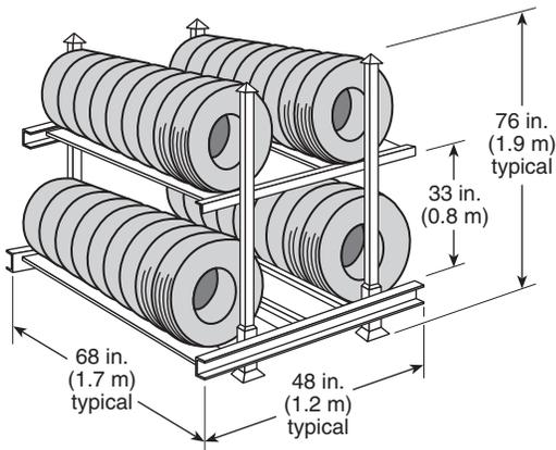
Figure 6-2(e) Palletized portable rack on-side tire storage arrangement (banded or unbanded).
