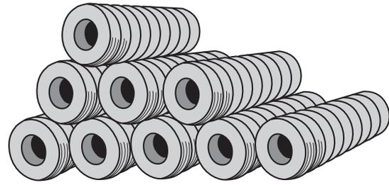
Figure 6-2(d) Double-row fixed rack tire storage.
