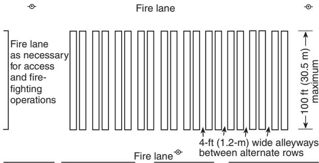
Figure E-4.3.1(b) Crib-style stacking into solid rows.
