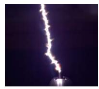
Tests have been performed according to IEC 60060-1 standard protocol. The insulation is greater than 97 %.
