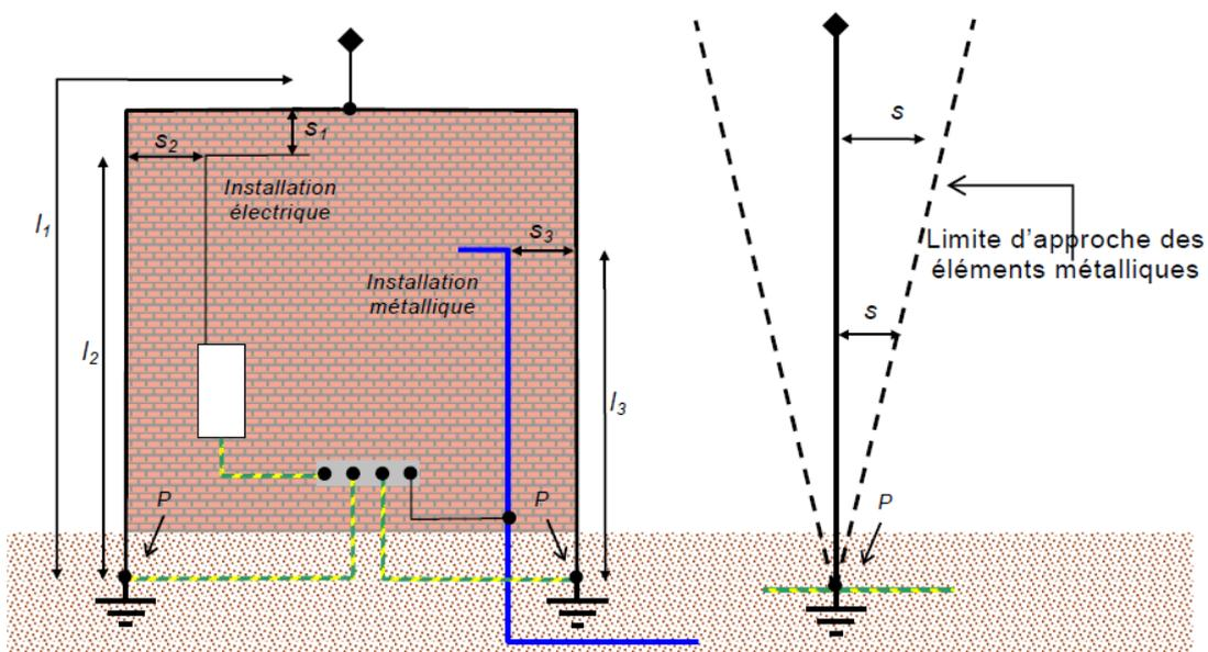
*Drawing of the separation distance according to the considered length*
