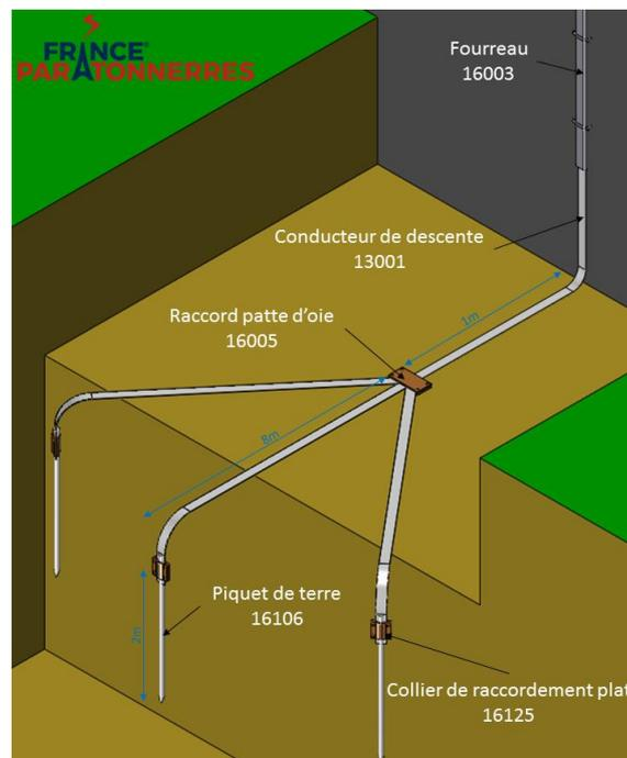
Example of an earthing system of Type A2, called « Triangle »
