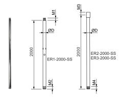
Stainless Steel Mast Used for Support Lightning Rods
